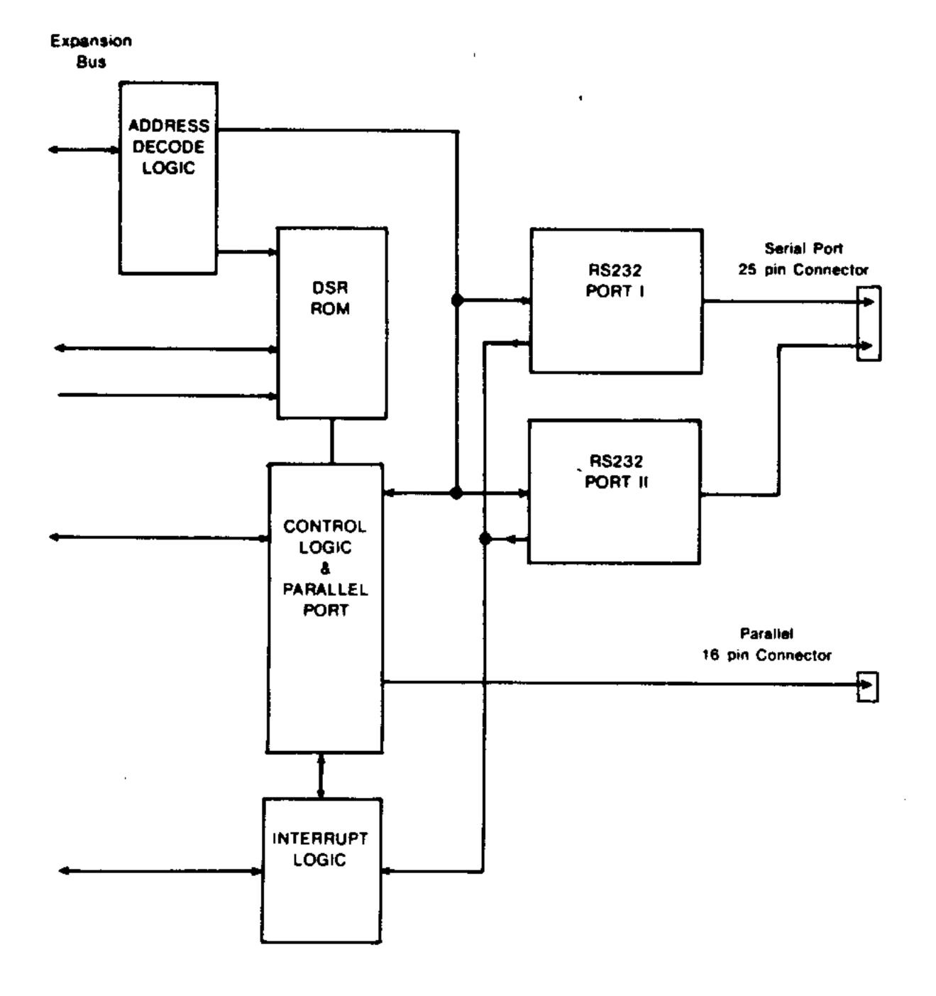
To change the CorComp card from RS232/1 and /2 to RS233/3 and /4 is very simple. Facing the card with the connector pointed to you, you can see the DSR-EPROM just in the middle of the card. (Type 2764. To the left ther is a jumper installed (J1) with 2 positions. Place the jumper on the 2 pins on the left (on my card marked with RS232 3,4) and from that moment it can and will operate as RS232/3 and RS232/4 and PIO/2. RS232, RS232/1, RS232/2, PIO and PIO/1 are now not longer available on THIS
